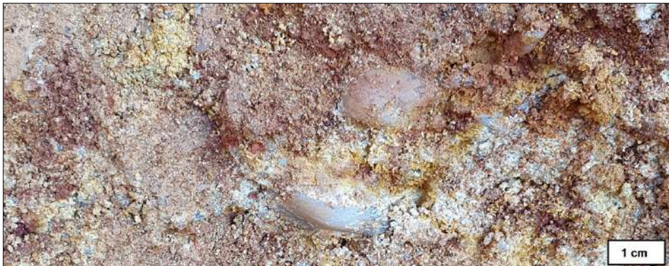
Figure 37 : Sediment 2 - clay-rich and quartz pebble conglomeratic sand. After Pelletier & Scodnick (2022).
