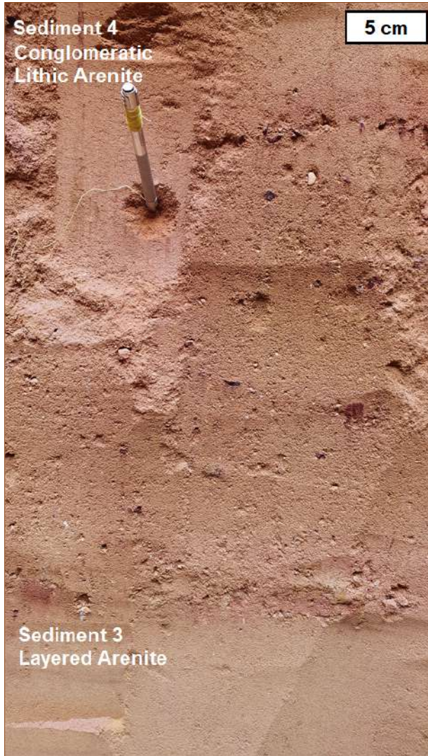
Figure 41 : Sediment 4 – micro-conglomeratic sand with minor iron oxides or hydroxides. After Pelletier & Scodnick (2022).
