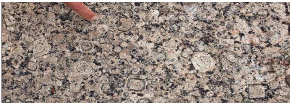
Figure 35 : Parguaza rapakivi granite showing medium to coarse grain orbicular texture. After Pelletier & Scodnick (2022).
